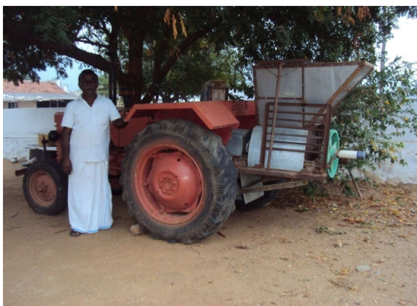
Tapioca stem grinder (Agricultural waste grinder) by Jayaprakash, Rasipuram
